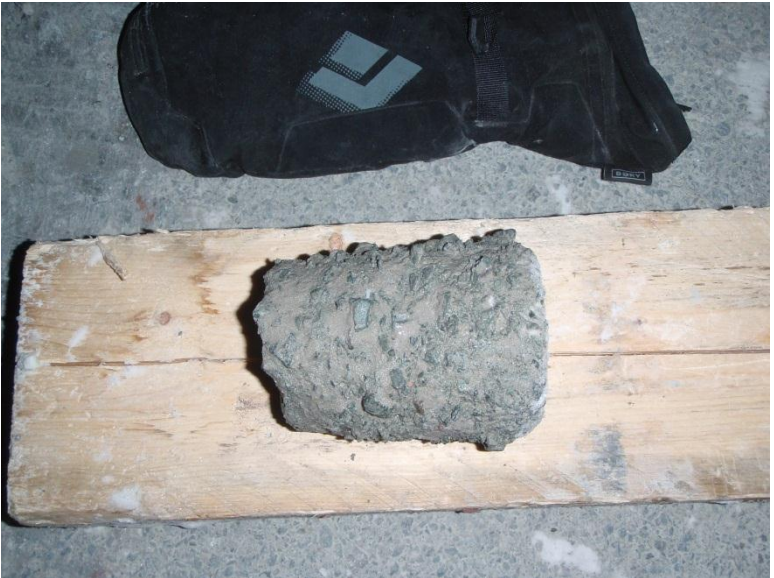
Photo 3: Drill core HB12-ND-CORE-DC22-QA-20120204. Poor quality due to gravel spinning during drilling. Some of the core broke off down the hole and was unable to be recovered.
